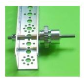
vii. Add Wheel Assembly with hub towards channel and tighten set screw over flat face of axle.
