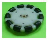
d. Place 2<sup>nd</sup> Omni wheel protruding hub over 1<sup>st</sup> wheel hub with rollers offset lining up 4 of the center holes. You will see light through 2 of the holes as 2 already have bolts installed – insert Omni bolts into these holes.
