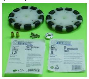
a. Using contents of Omni wheel bag plus (2) Bronze Bushings [39091] press bushing into center of each wheel hub – this is a tight fit & will need very strong fingers or a rubber mallet.
