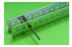
v. Slide Gear Assembly from step 1b over axle flange side leading and screws away from channel then tighten set screw over flat face of axle.
