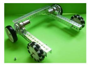
h. Slide 2<sup>nd</sup> set collar over axle and tighten set screw over flat face of axle. Make sure all pieces are pushed together with no slack and Dually Assembly is on outside of frame.
