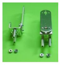
c. Attach phone holder assemblies with (4) 6-32 socket head cap screws ½" long [39098] to back of robot through 64 x 192mm Flat Building Plate [39073] & top of 288mm Channel [39068]. Line phone holder brackets with adhesive backed foam to cushion phone.
