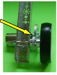
d. If 40 tooth and 80 tooth gears do not perfectly mesh – grab motor in one hand and side rail in other hand and rotate motor towards long end of side rail. If this does not correct the gear mesh try rotating motor the opposite direction.
