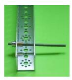
iv. Slide 2<sup>nd</sup> bushing over axle leading with non-flange end so that bushings are mirror images on axle.
