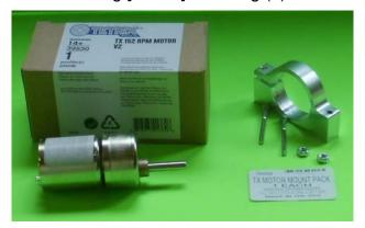
i. Push Motor Mount onto the axle side of the Motor which is a tight fit, requiring two people, one to spread open the mounting bracket while the other pushes the motor into place. The mounting bracket will set itself into a depression in the motor casing. The screw opposite the motor axle should be slightly above the bracket gap. BE CAREFUL NOT TO BREAK PINS ON OTHER END OF MOTOR.
